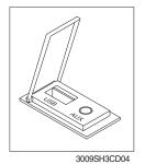
(1) MP3 files are played when a USB device is connected to the USB port.
