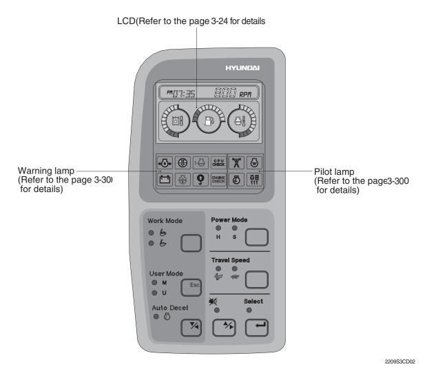
\* The warning lamp lights ON and the buzzer sounds when the machine has a problem. In this case, press the buzzer stop switch and buzzer stop, but the warning lamp lights until the problem is cleared.
