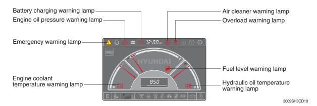
Each warning lamp on the top of the LCD pops up on the center of LCD and the buzzer sounds when the each warning is happened. The pop-up warning lamp moves to the original position and blinks when the select switch is pushed. And the buzzer stops. Refer to page 3-10 for the select switch.
